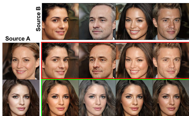
Fig. 18 Style mixing. The source A and B images are generated from input latent codes z_A and z_B . The images in the red box are generated by applying the w_B (the intermediate latent corresponding to z_B ) to G_s and w_A (corresponding to z_A ) to G_d . The images in the green box are generated by applying the w_A to G_s and w_B to G_d (Color figure online)
