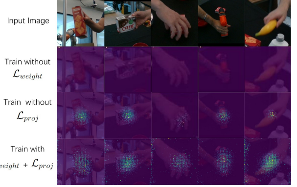
Fig. 9: Attention maps of 512 query points on the shape prior. The bright areas indicate the high probability to be an object.
