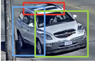
Figure 4. The part detection results. The red bounding box indicates the top part, and the blue box and green box indicate the side and front part respectively.
