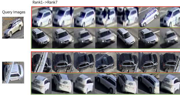
Figure 6. Visualization of matching results with and without part-aware verification. The first and the second row for each query are the matching results without and with part-aware verification respectively.
